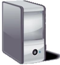
**Computer case:** The case that holds all the electronic components of the computer. On the outside of the case is where you can plug in headphones, microphones and USB devices. These ports are usually found on the front of the case. The ports for network cables, printers and power cords are usually found in the back.
